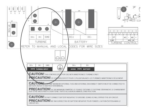
Figure 2.5 Turbine Connection Location
